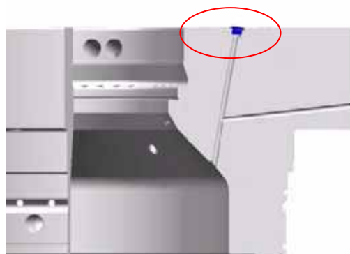
Substitute the safety valve with a plug in accordance with EN47AR22 Add a jacketed packing ring in accordance with EN14B2230
